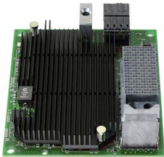
Figure 1. IBM Flex System CN4058 8-port 10Gb Converged Adapter
